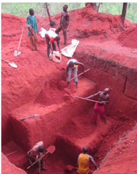
**SMARTER mining combines 'stepping' with 'trenching' to improve productivity and mitigate environmental damage. In this trench, workers move the diamond-bearing gravel up the steps into bags.**
