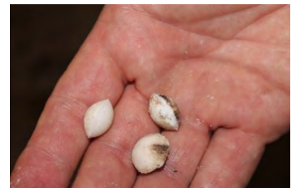
Figure 7: After calibrating the briquette machine the perfectly formed 1.8g Urea briquette were produced.
