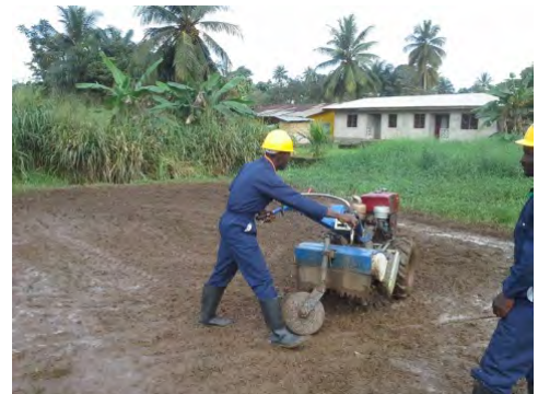
Figure 8: One of the participants demonstrates the use of the power tiller during training in Lofa County.
