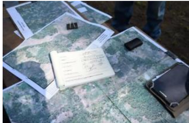
The core set of tools for delimitation including tablet, GPS device, satellite imagery, and receipt book ILRG MOZAMBIQUE 25
